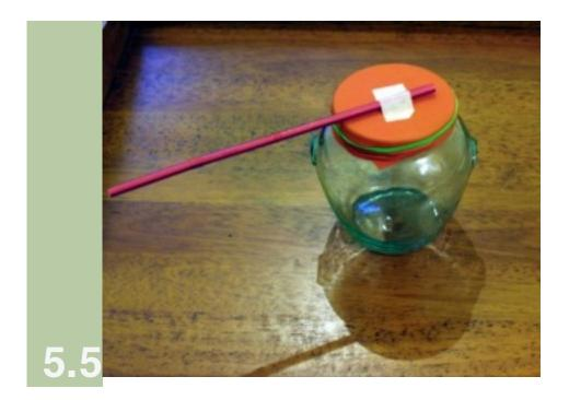
Tape the straw onto the balloon lid; the straw should be sitting one quarter of a way on the lid, with the tape about 2 cm or 1 inch from the edge of the straw end that is sitting on the balloon lid. The straw is your indicator "needle". Trim the straw if it's too long, but leave more length off the jar as what is attached to it.
