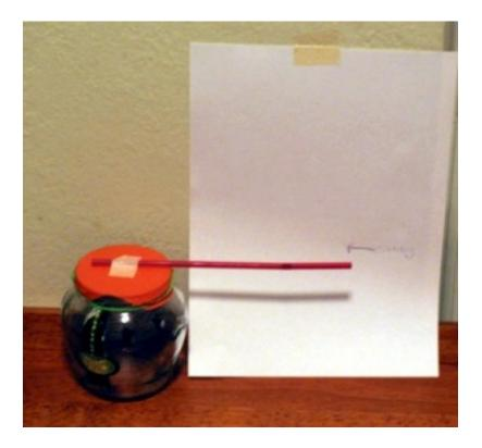
Put the finished glass jar next to a wall and tape a piece of paper or card to the wall behind it.
